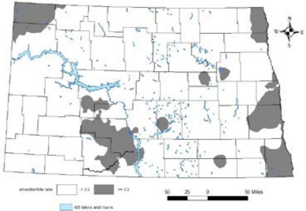
Figure 3. Smectite-to-illite ratio of surface soils in North Dakota from a soil sampling conducted in spring 2017. Dark gray regions are greater than 3.5. White areas are less than 3.5.
